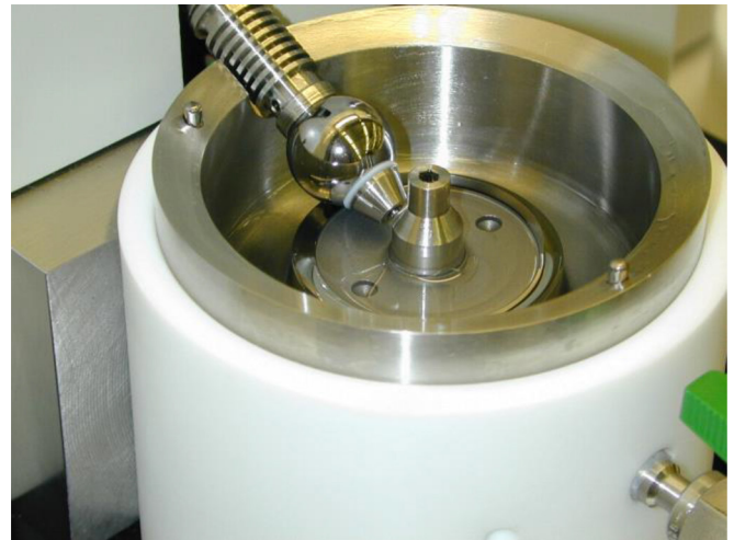
Figure 1. MTM test showing highly loaded contact used in this study to measure EHD friction.
