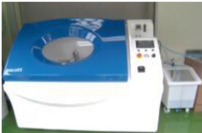
Figure 4. Cyclic corrosion test chamber
