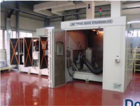
Figure 3. The brake dynamometer of vehicle scale
