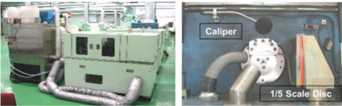
Figure 2. (1) 1/5 Scale dynamometer external structure. -left (2) Internal structure. -right
