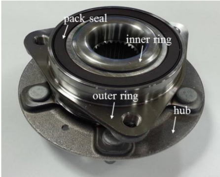
a. Configuration of automotive wheel bearings
