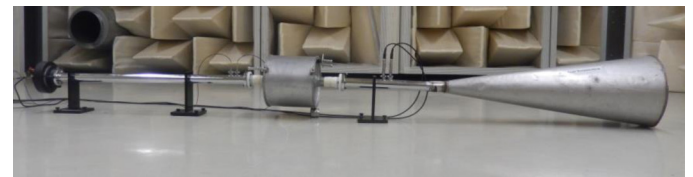
Figure 8. Transmission Loss measurement set up with anechoic termination [reproduced with permission from M/s Sharda Motors Ltd.]
