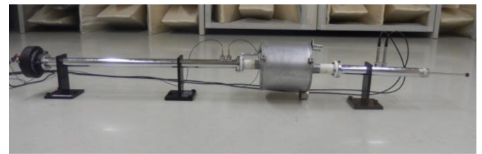
Figure 7. Transmission Loss measurement set up with rigid load termination [reproduced with permission from M/s Sharda Motors Ltd.]
