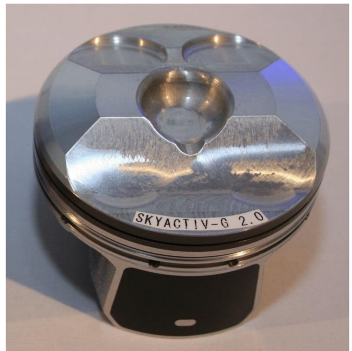
Figure 3. Piston of a Mazda skyactive engine with central cavity. [13]
