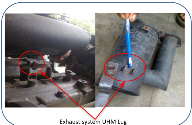
Fig.3. Photograph of UHM Lug failure
