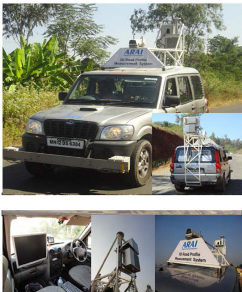
Figure 4. 3D Road scanning system fitted on ARAI test vehicle
