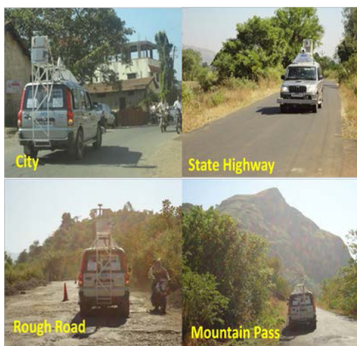
Figure 5. ARAI 3D road profile measurement vehicle on different routes
