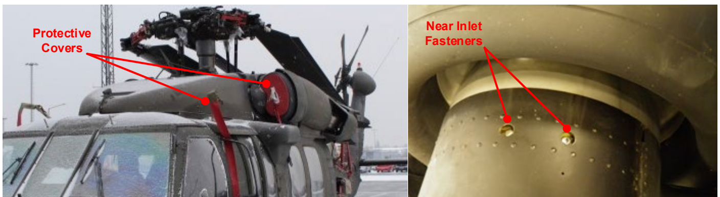
Figure 2 - Examples of possible sources of installation FOD (Source: U.S. Army)
