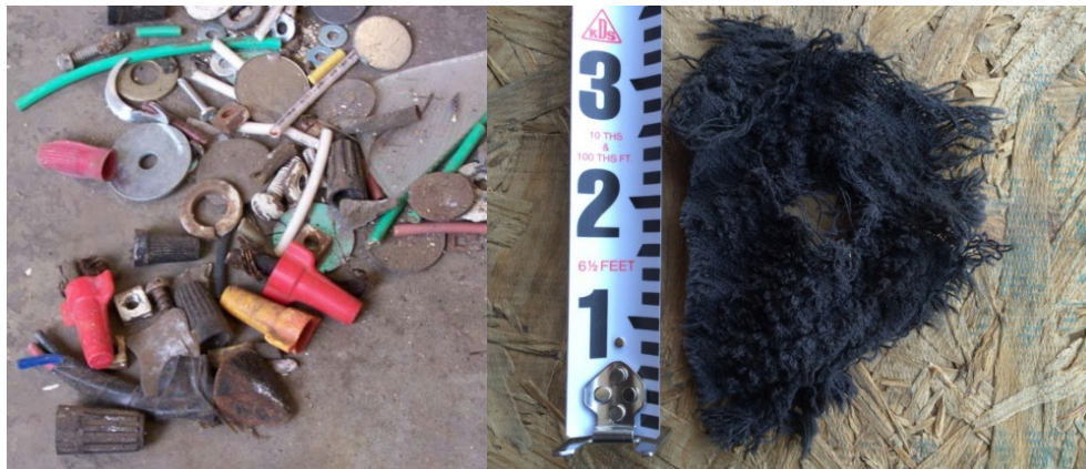
Figure 3 - Examples of maintenance FOD (Source: NASA and NTSB)
