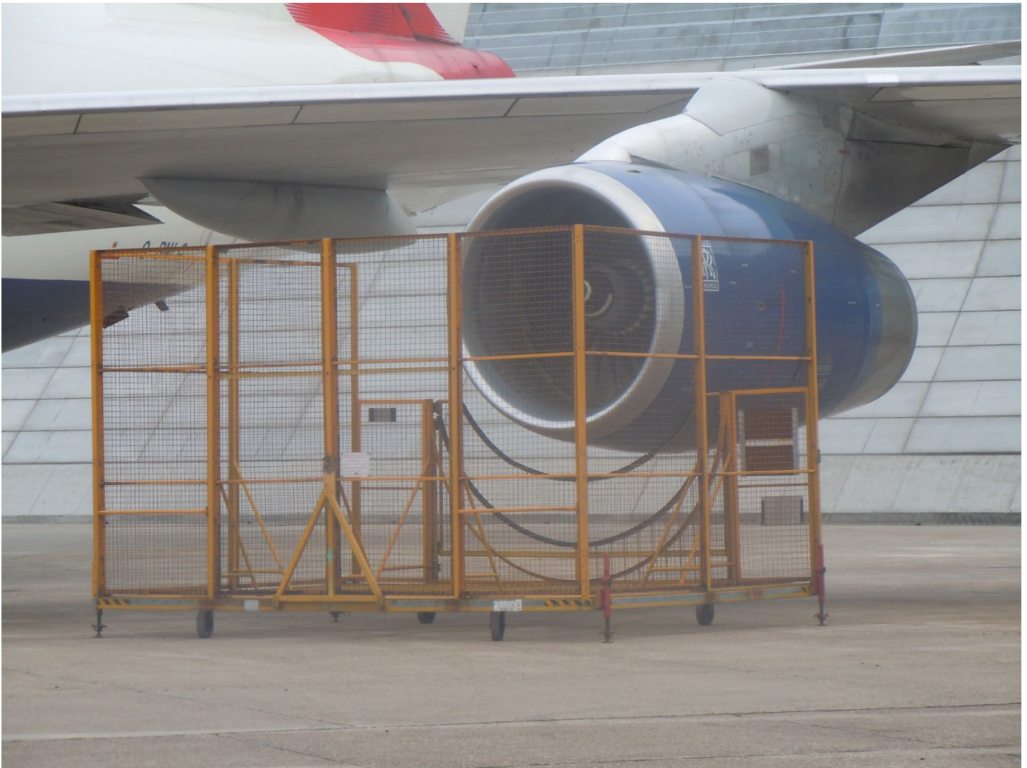
Figure 4 – Fod guard incorporating anti vortex floor mesh
