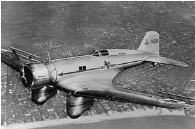
Figure 15 - Northrop Gamma 2 had landing gear with streamlined coverings that extended down from the fuselage with the wheels protruding from the bottom
