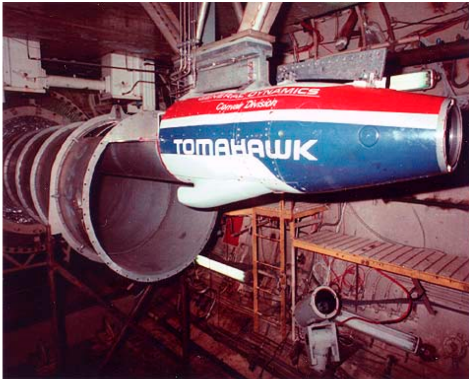
FIGURE 5 - TOMAHAWK INLET/ENGINE MODEL IN AEDC TEST CELL J-1, REAR QUARTER VIEW
