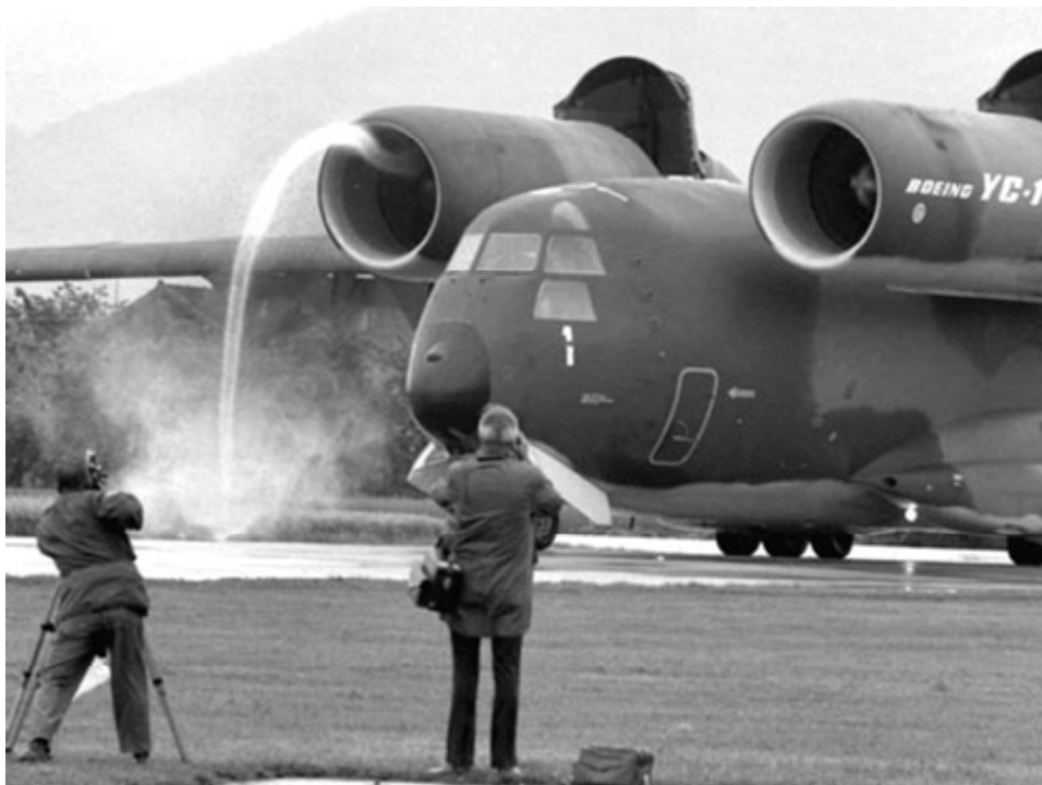
FIGURE 21 - PHOTOGRAPH OF A TIGHTLY-WOUND GROUND VORTEX DURING THRUST REVERSER OPERATION
