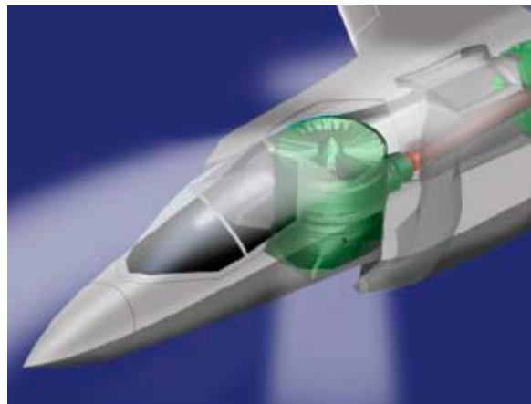
FIGURE 8 - LIFT FAN INSTALLATION IN F-35B JSF
