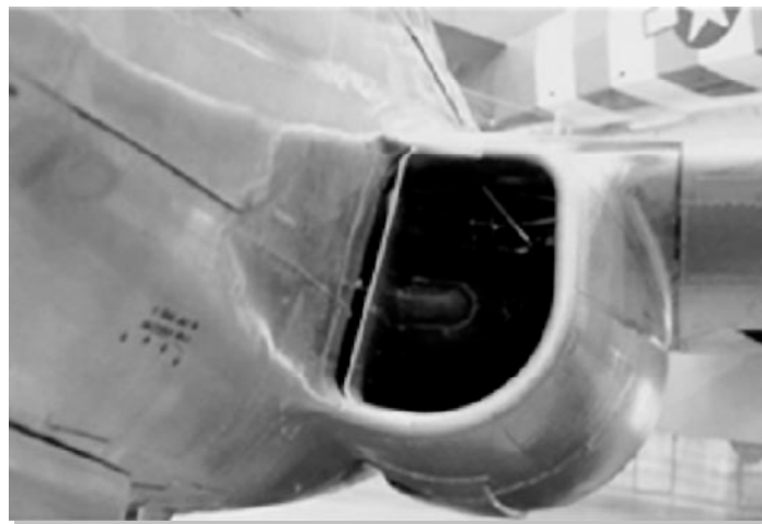
FIGURE 1 - INLET INSTALLATION OF THE BELL P-59
