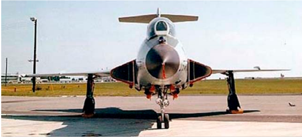
FIGURE 6 - F-101 INLET CONFIGURATION WITH EXTERNAL DIVERTER AND SIDEPLATE
