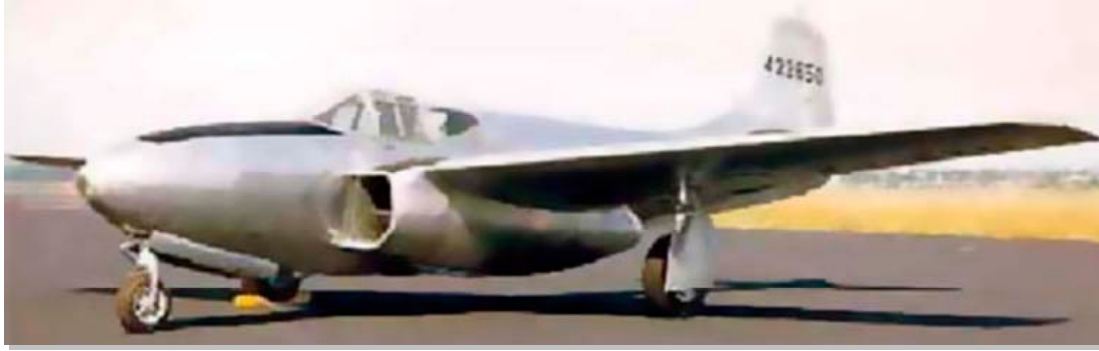
FIGURE 1 - INLET INSTALLATION OF THE BELL P-59
