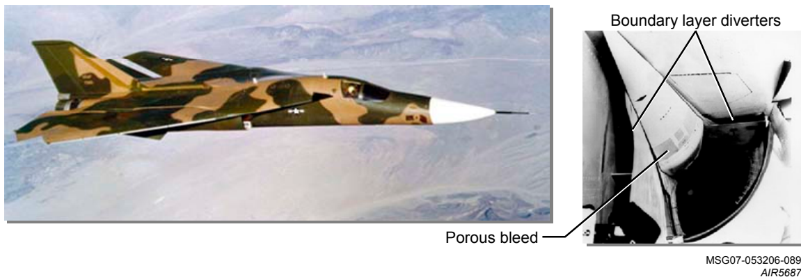
FIGURE 7 - INLET SYSTEM FOR THE F-111
