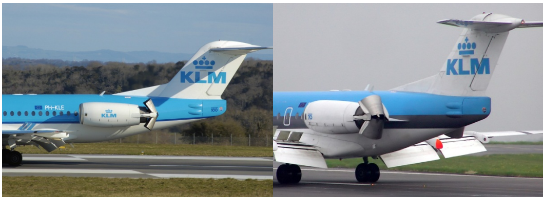
Figure 10 - Target thrust reverser installation on KLM FOKKER 70
