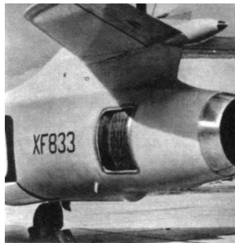
Figure 5 - Thrust reverser installed on a Hunter 6 aircraft (Reproduced from Reference 10)
