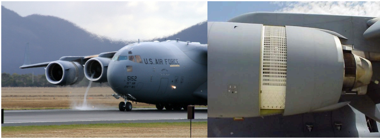
Figure 15 - Cascade thrust reverser with translating fan cowl installed on the C-17 (left photo by Alastair Bor)
