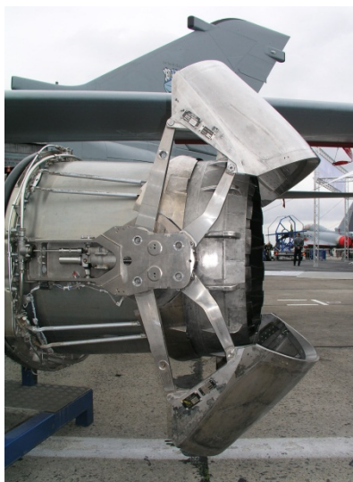
Figure 11 - Target thrust reverser installed on Rolls-Royce RB199 engine (Photo by Remy Blot)
