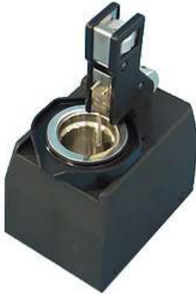
Figure 9 - Typical ultrasonic cleaner for optical fibers (courtesy AFL)
