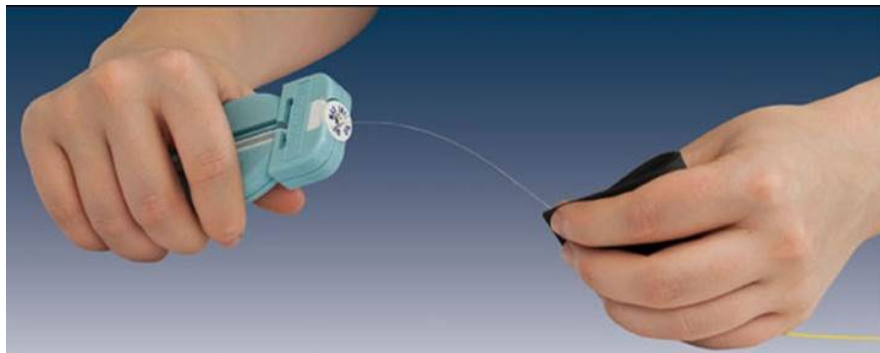
Figure 6 - Removing 250 \mu\text{m} acrylate primary coating (courtesy Thorlabs)
