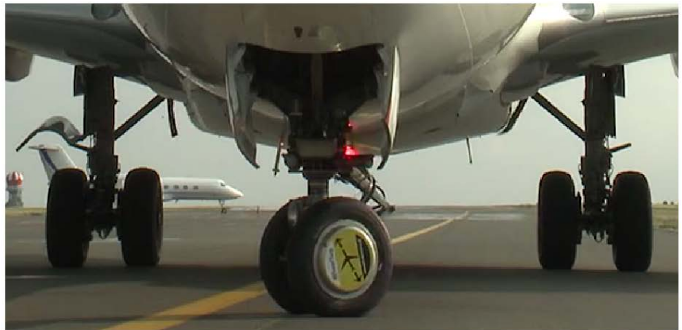
Figure 7 - Boeing 737NG caster angle
