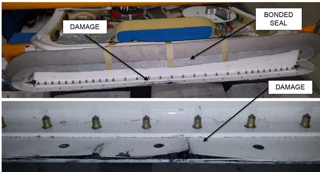
Figure 9 - Damage resulting from removing a bonded pressure seal on a pax door
