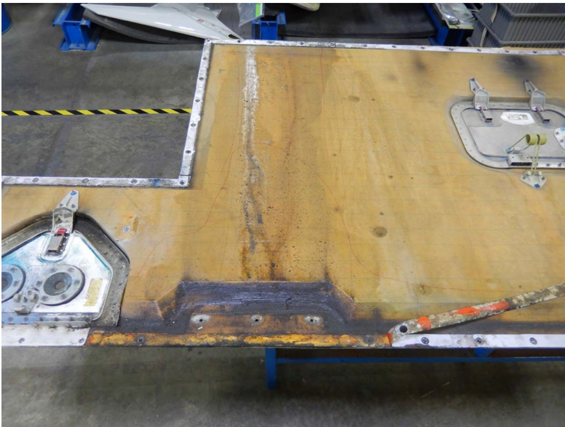
Figure 13 - Example of sandwich panel contaminated by hydraulic fluid
