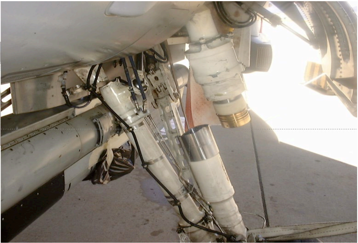
Figure 1 - Representative landing gear part with hydrogen embrittlement failure
