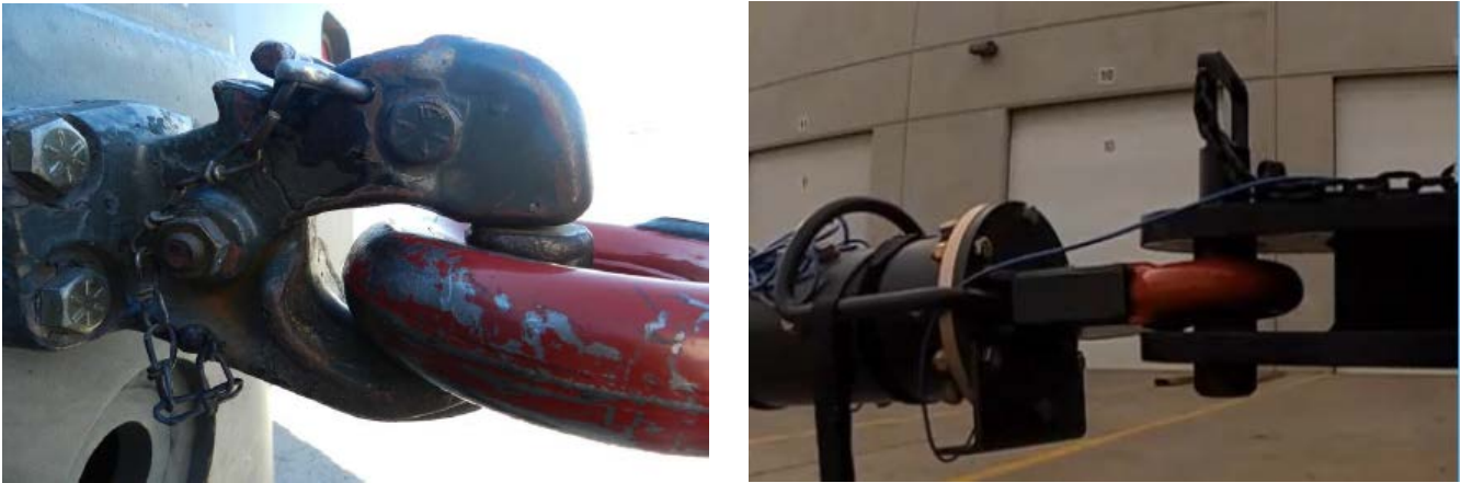
Figure 2 - Pintle and pin and clevis hitch-tow interfaces
