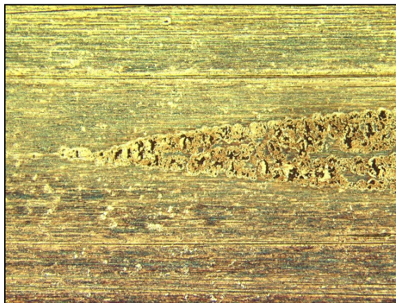
Figure 1B - Micropitting evidence caused by surface imperfection, 50x
