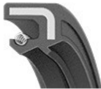
Figure 3 - Elastomer rotary lip seal, case molded over
