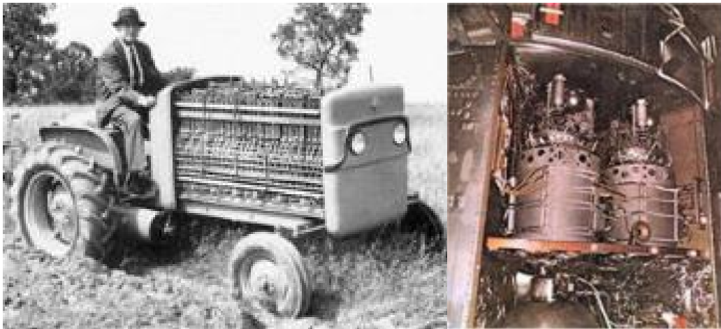
Figure 5 - First ever hydrogen fuel cell vehicle in 1959; NASA's gemini spacecraft fuel cell in 1962
