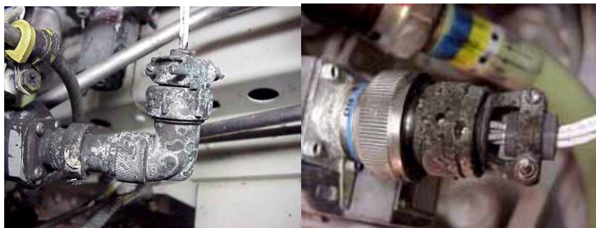
Figure 1A - Corroded aircraft connectors that had ionic contamination attributed to deicers
