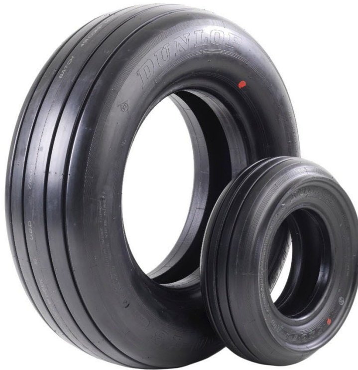
Figure 1 - Non-chine main landing gear tire next to a single-chine nose landing gear tire Reprinted with permission. © Dunlop Aircraft Tyres Limited.
