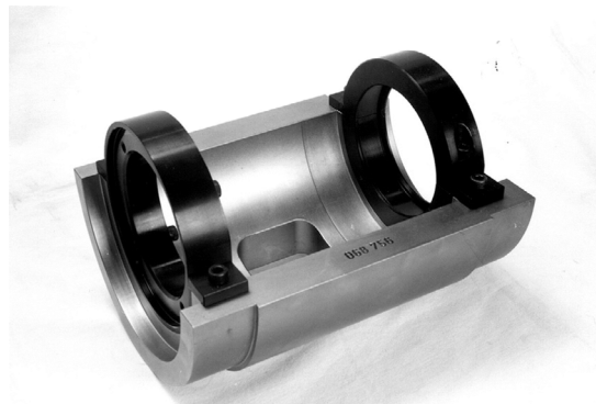
FIGURE 7 - Cradle for Horizontal Balancing Machine
