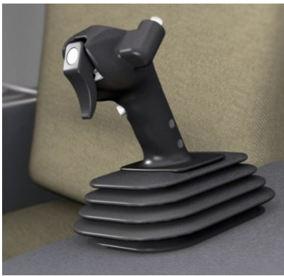
Figure 4 - Typical installation of a side stick in the pilot's side console
