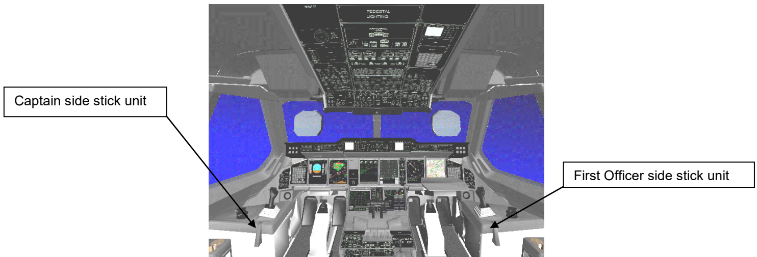
Figure 3 - Typical location of the side sticks in a flight deck
