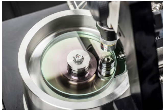
Figure 4 - PCS Instruments EHD Test Instrument - close up of test chamber for film thickness test
