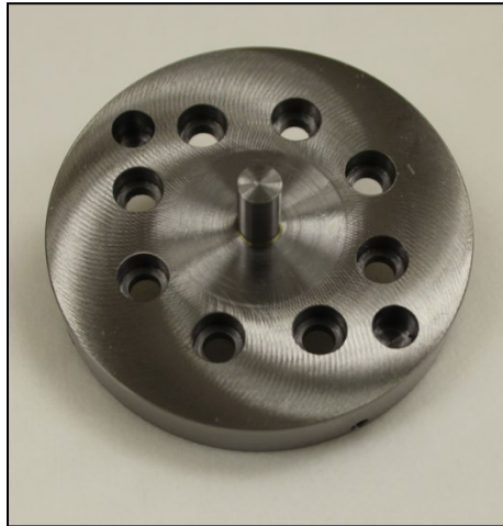
Figure 11 - Driven ball optics nosepiece adaptor
