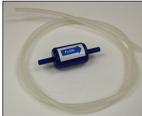
Figure 13 - Silicone tubing and inline oil filter
