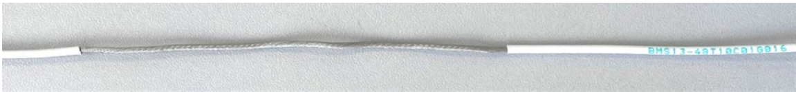
Figure 1 - Example of single core wire with skin splice
