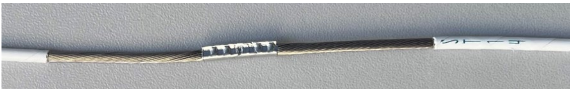
Figure 3 - Example of single core wire with uninsulated crimped butt splice
