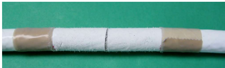
Figure 2 - Application of PTFE protective tape
