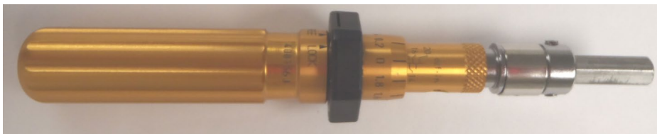
Figure 1 - Torque wrench with torque adapter bit for use on MIL-PRF-29504/5 termini
