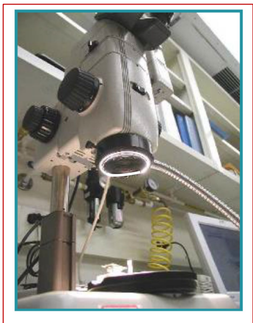
Figure 5 - Ring lamps tend to inhibit whisker detection due to excessive glare from background or adjacent surfaces
