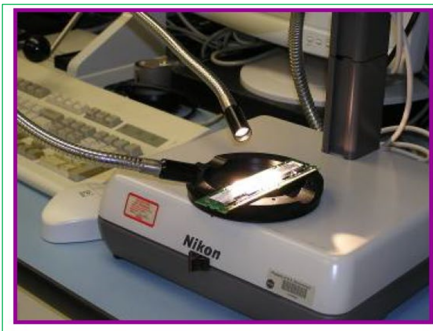
Figure 6 - Directional LED lighting with narrow beams increases probability of whisker detection due to control of the angle of illumination
