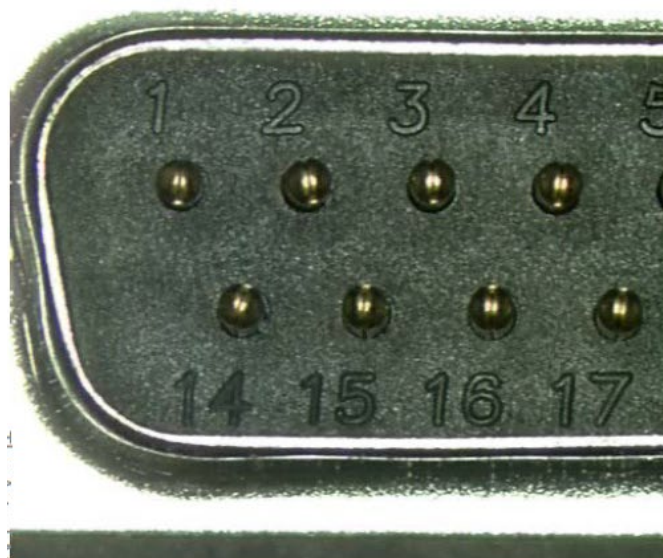
Figure 7 - Ring lamp illumination of tin-plated connector shell results in excessive glare compared to whisker illumination (compare with illumination on right)
