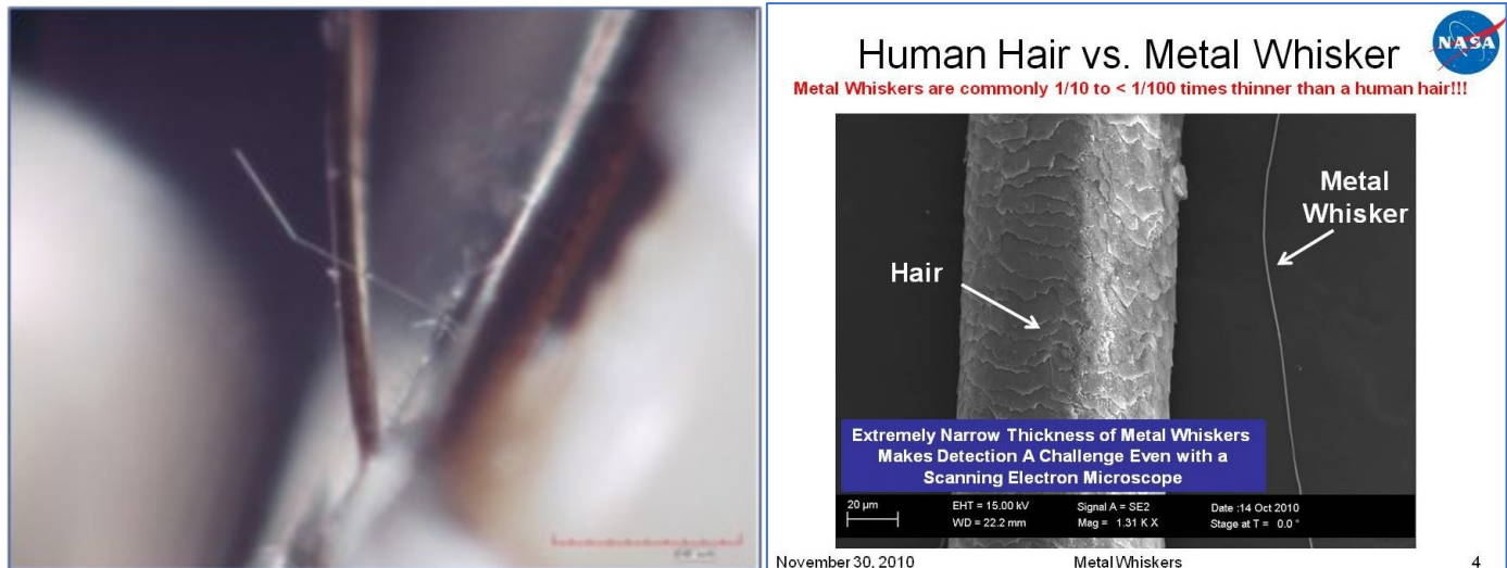
Figures 2 and 3 - Optical and SEM images comparing the thickness of a metal whisker to a human hair
