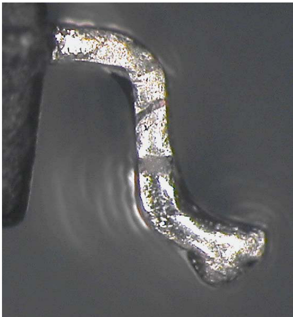
Figure 1G - Excessive, uneven, or poor plating (left image courtesy of Silicon Cert Laboratories, LLC; right image courtesy of Honeywell)
