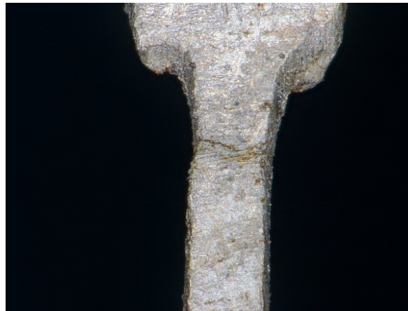
Figure 1D - Repaired leads (Image courtesy of Honeywell)
