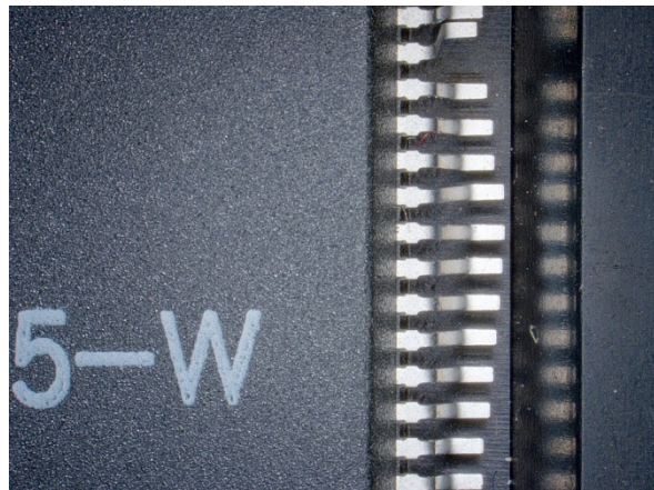
Figure 1E1 - Bent or noncoplanar leads (Images courtesy of Honeywell)
