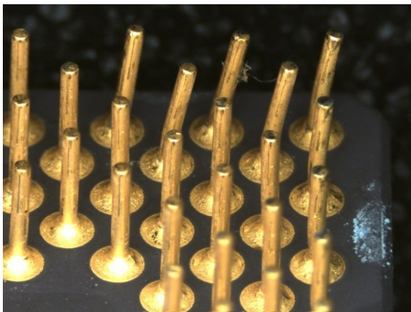
Figure 1E1 - Bent or noncoplanar leads (Images courtesy of Honeywell)
