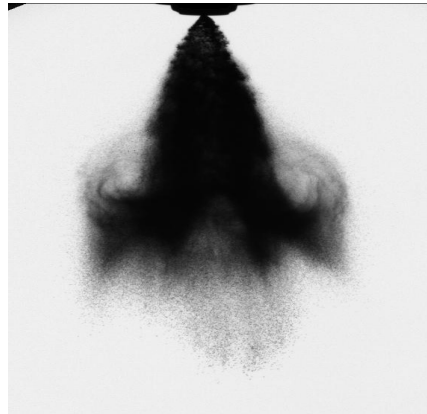
FIGURE 5 - TYPICAL BACK-LIT IMAGE OF A G-DI SPRAY
