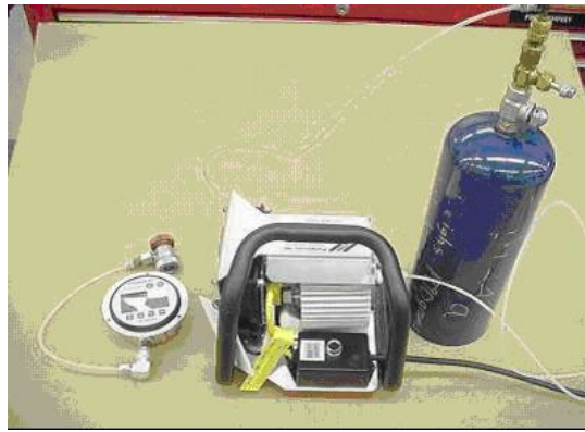
Figure 1 - Recovery vacuum pump and cylinder used in laboratory refrigerant recovery procedure
