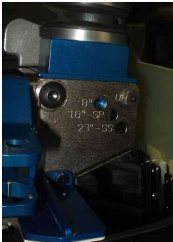
Figure 9 - Right view showing neck angles achieved when placing adjusting shoulder bolt in different positions
