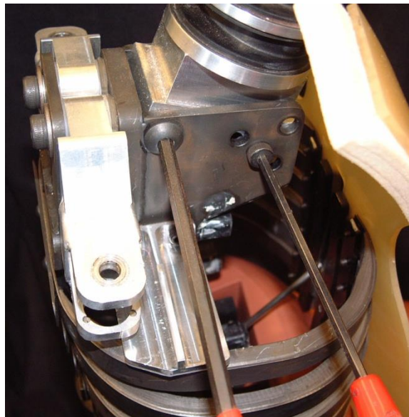
Figure 8 - Right BHCS and adjusting shoulder bolt attaching neck assembly to spine box
