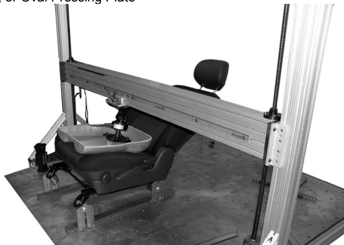
FIGURE 1 - EXAMPLE STATIC LOAD DEFLECTION TEST EQUIPMENT
