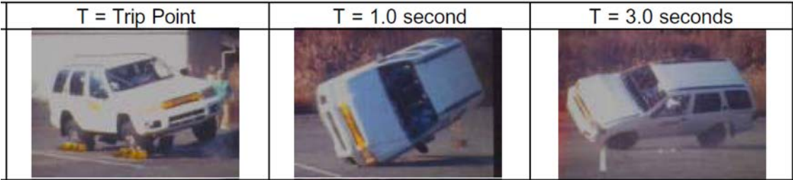
Figure 10B - Example of tripped rollover procedure runs
