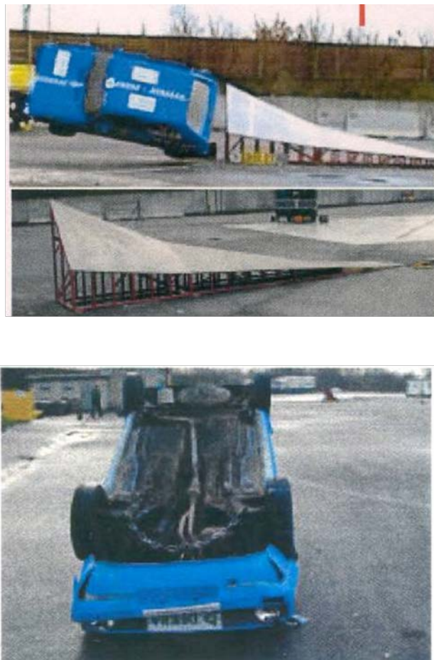
Figure 8 - Corkscrew test mode using spiral ramp
