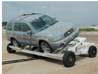
Figure 1A - Close up of J2114 dolly rollover fixture (courtesy of Exponent)
