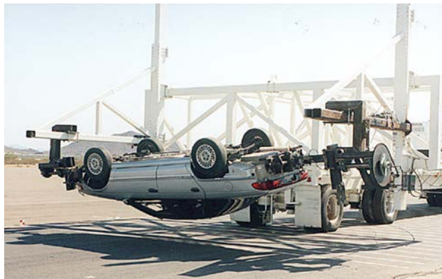
Figure 2 - Test vehicle and fixture for CRIS procedure test
