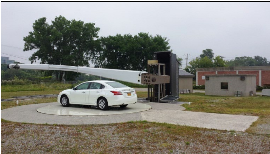
Figure 10 - Example facility for collecting data from DSRC transmit coverage tests
