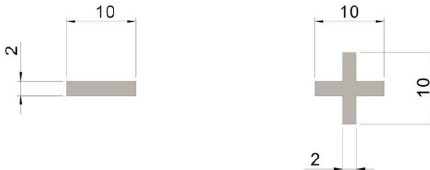
Figure 1 - Marking of polarity (millimeters)
