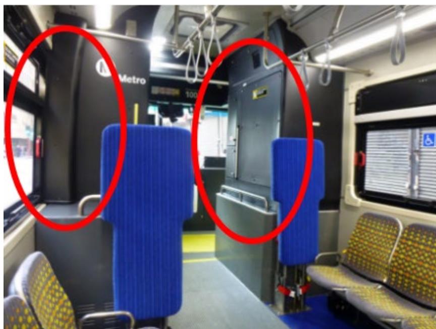
Figure 1B - Battery packs located on the front wheel houses Source: Riley, on Flickr
