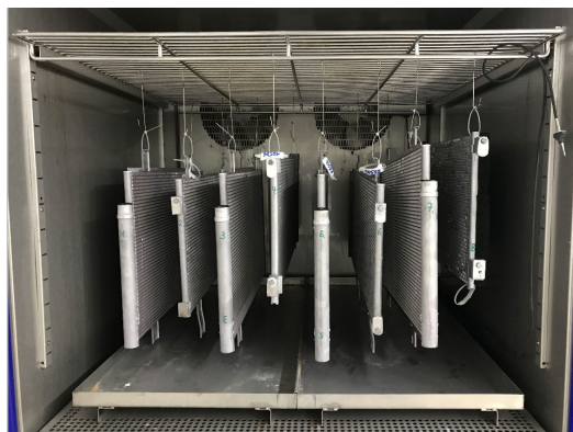
Figure 7 - Example of test position of the components in the cyclic climate test chamber
