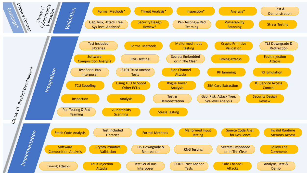
Figure 1 - V&V methods to ISO/SAE 21434 mapping relationship
