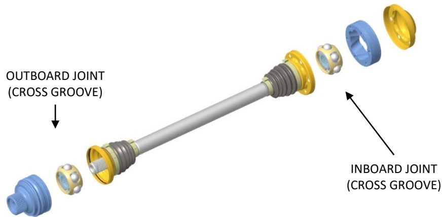
Figure 7 - Typical rear-wheel-drive halfshaft with end motion constant velocity joints (cross groove type shown)
