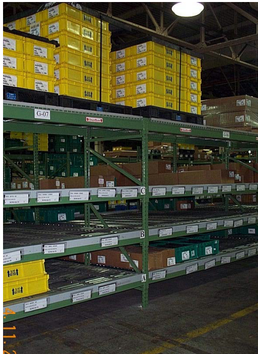
The loading end of the roller rack in the Marketplace. In this picture, there is an extra level of storage for extra inventory, and this stock is accessed using motorized lifting equipment.
