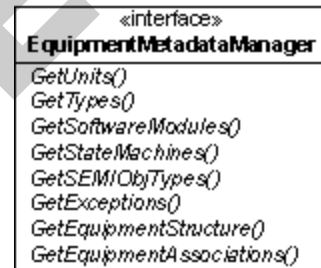
Figure 2 Interface for Accessing Equipment Metadata
