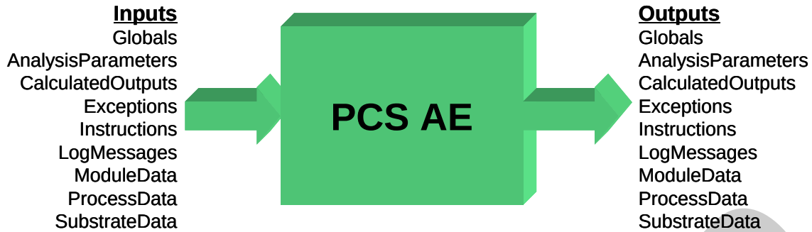
Figure 2 PCS Analysis Engine Common Input/Output Structure
