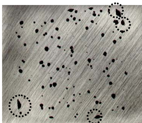
Figure 2 Examples of Crevice Corrosion (Dashed Circles) on Type 316 Stainless Steel After a Pitting Potential Test in 1 M NaCl 2 (11× Magnification)
