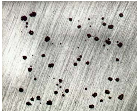
Figure 1 Examples of Pitting on Type 316 Stainless Steel After a Pitting Potential Test in 1 M NaCl (11× Magnification)
