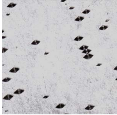
Figure 2 Dislocation Etch Pits on (110) Silicon, Following 5-Min Wright Etch, Magnification 110×
