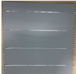
Figure 2 Specimen After Back Electrode Soldering
