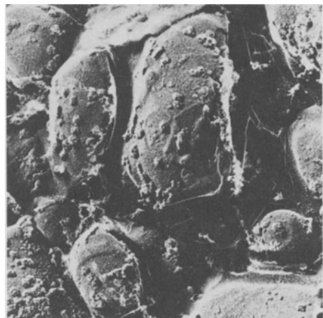
Fig. 5.1 — Intermetallic compound crystals with inclusions at surface which have formed during soldering of copper cleaned with fine abrasive
