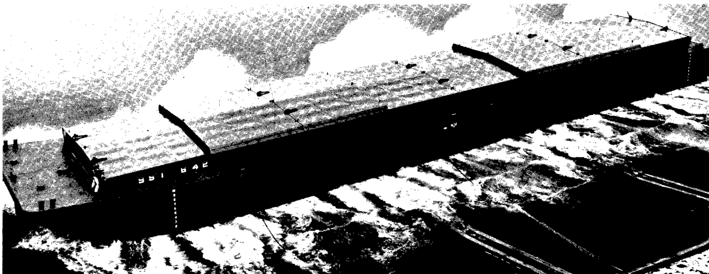
FIGURE 1 Covered hopper barge. Covers roll away to expose cargo compartment.
